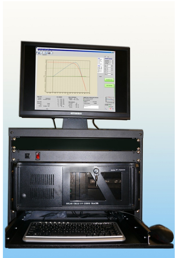
Figure 3: Typical I-V System Console – 15A/20A Current
